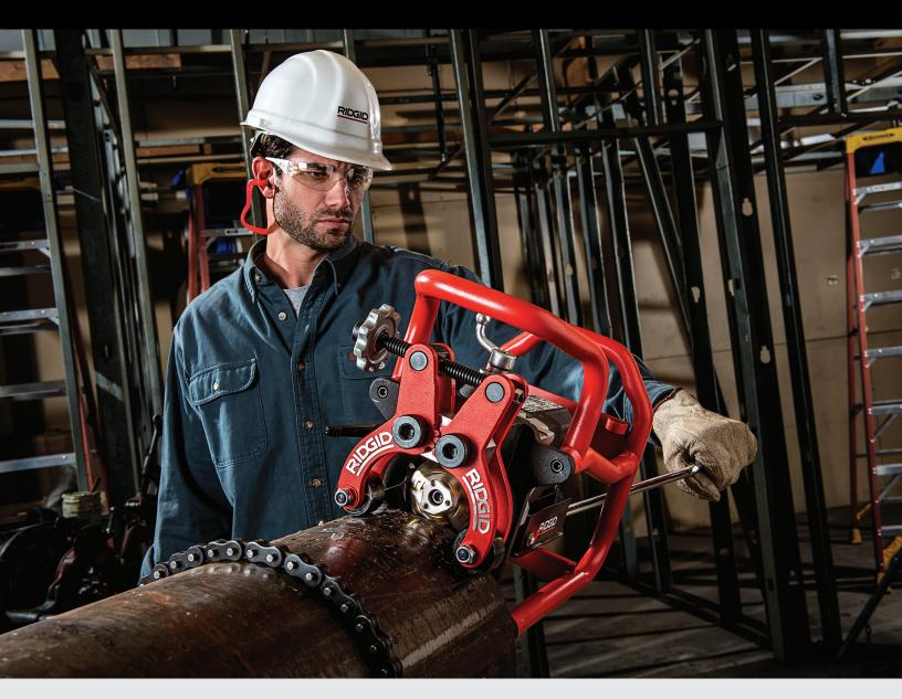
Set-up and bevel 12" diameter schedule 40 pipe in one pass in under 2 minutes using the new B-500 Transportable Pipe Beveller. (Pipe capacity: 4" diameter and larger, 3/16" - 1/2" wall - See Specifications.)
